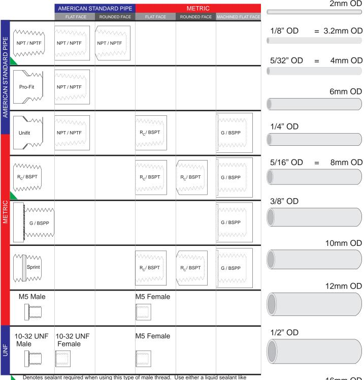
Denotes sealant required when using this type of male thread. Use either a liquid sealant like Loctite® 545, Teflon® tape, or pre-applied sealant that can be ordered already applied to many pneumatic fittings.
