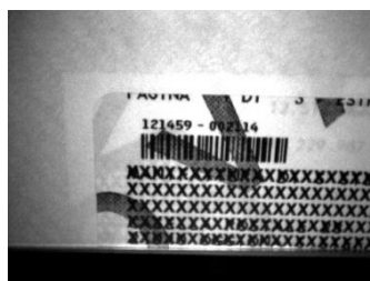
Figure 22 - Overprinted Barcode Readable by Matrix 210N also Through the Envelope Window Film
